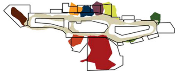
Fig. 22. Constructed floor plan of story 2 by CrowdInside++, which has several artificial improvements that are not always possible in reality.
